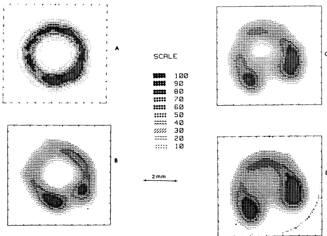
Fig. 6: Time dependent EPR images of polycarbonate (5.8 mm I.D. x 60 mm length rod) after solvent swelling in 5-10 mM TEMPOL (10% water/90% DMF) for the period shown: A, 12 hrs., B, 24 hrs., C, 72 hrs., D, 96 hrs. From Berliner, Wan and Fujii, 1986, with permission.
