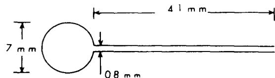
Fig. 1: The single turn, flat loop coil. Dimensions of the loop were 7 mm O.D., 41 mm length, and 0.8 mm gap. The loop was made of 0.7 mm (O.D.) insulated copper wire. (From L.J. Berliner and H. Fujii (1985) with permission).
