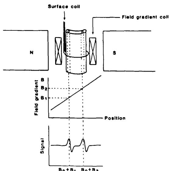
Fig. 2: Diagram of the one-dimensional EPR imaging experiment of a celery sample soaked in 1 mM TEMPOL. The two capillaries were aligned along the z-field gradient direction.  $B_0$  is the applied magnetic field and  $B_1$  and  $B_2$  represent the static field contribution due to the field gradient at capillary positions 1 and 2, respectively. (From Berliner and Fujii, 1985, with permission).
