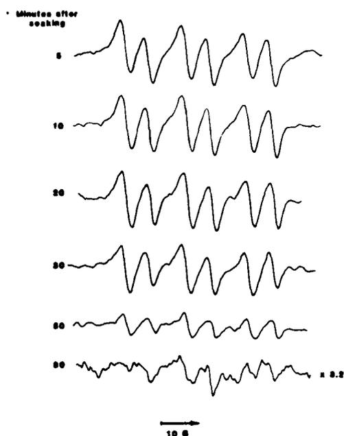
Fig. 3: Time dependence of the one-dimensional EPR spectrum of celery soaked in 1 mM TEMPOL. The z-gradient was 24.3 G/cm. Microwave frequency was 1.83 GHz; applied magnetic field, 0.0660 tesla; applied microwave power, 100 mW; and modulation frequency, 100 kHz. The two capillaries were 2.6 mm apart (center to center). After 50 minutes image resolution deteriorated with capillary breakdown and lateral diffusion of the nitroxide imaging agent. (From Berliner and Fujii, 1985, with permission).
